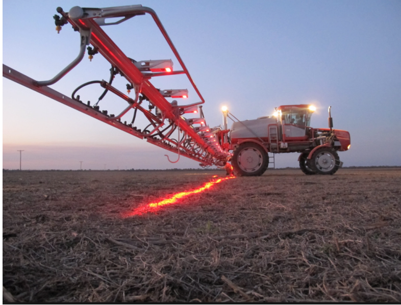
Figure 2.1: WEEDit configuration on a common sprayer (Romertron 2016)
